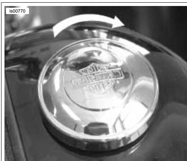
Figure 1. Right Hand Threaded Fuel Cap Installation
