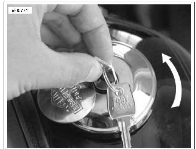
Figure 2. Right Hand Threaded Fuel Cap Removal
