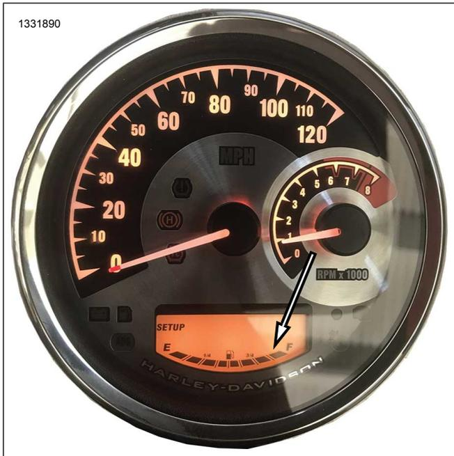
**Figure 3. Fuel Level Display Setup**
