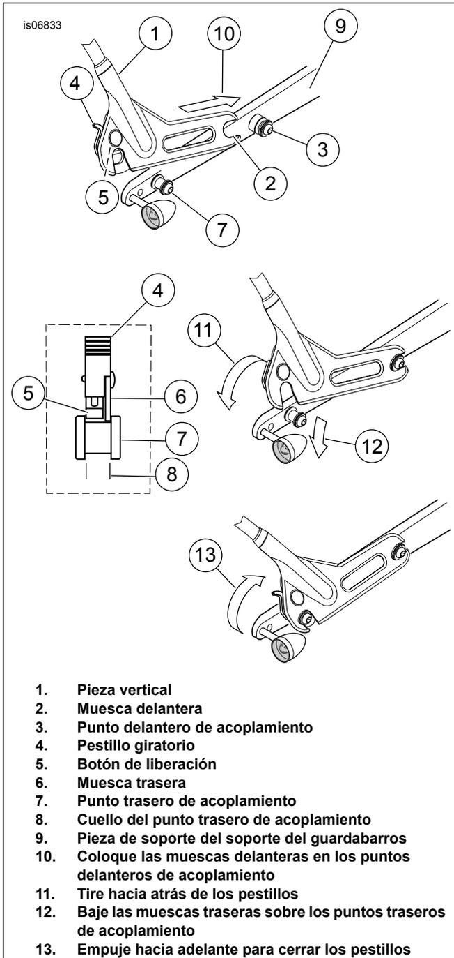
Figura 1. Pieza vertical desmontable
