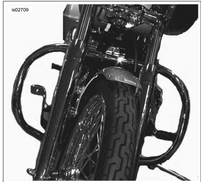
Figure 2. Engine Guard Installed
