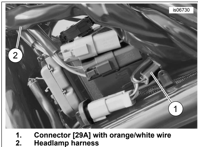
Figure 22. Wire Splice Locations (2004 V-Rod)
