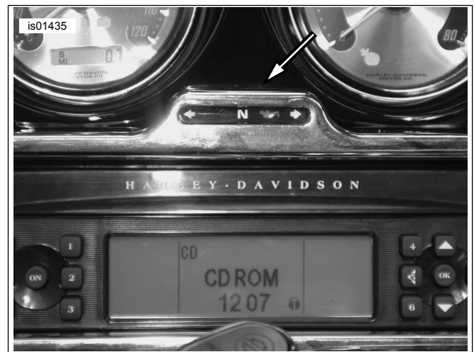
Figure 1. Indicator lights properly aligned through faceplate
