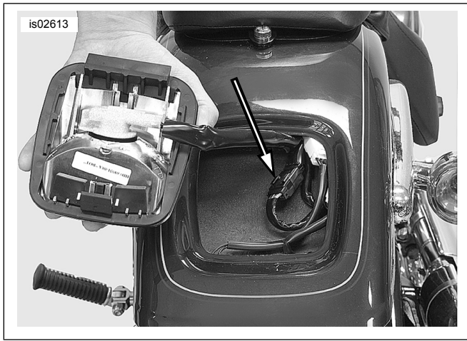
Figure 2. Tail/ Stop Lamp Wiring
