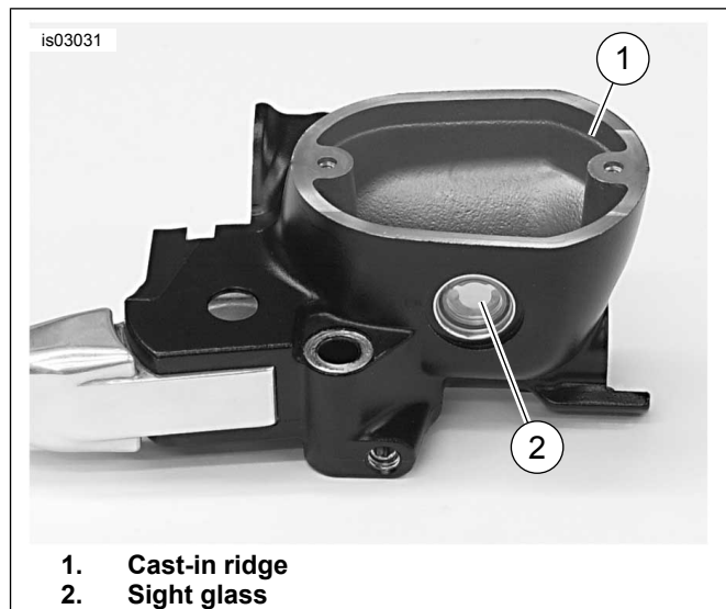
Figure 7. Filling Front Master Cylinder Reservoir
