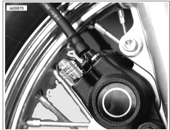
Figure 3. Installed Banjo Bolt Cover
