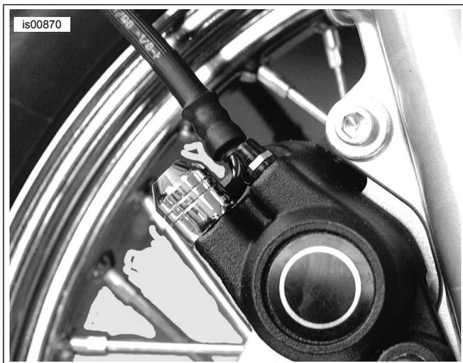
Figura 3. Tampa do parafuso banjo instalada
