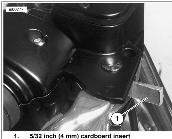
Figure 2. Brake Lever / Lever Bracket Cardboard Insert
