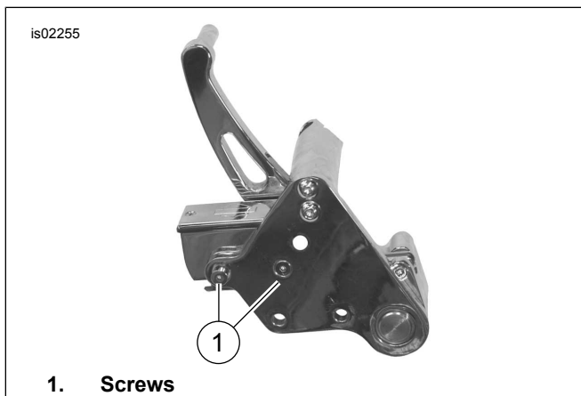
Figure 17. Secure Master Cylinder to Brake Plate Screws
