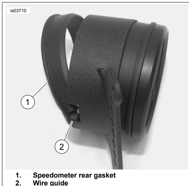
Figure 4. Remove Rear Speedometer Gasket (Shown with Wiring and Connector Removed)
