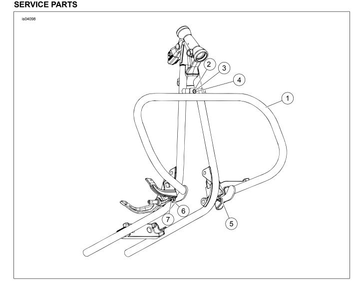
Figure 4. Service Parts: Black Engine Guard Kit
