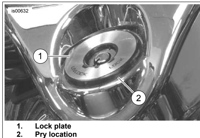
Figure 1. Remove Fork Lock Plate
