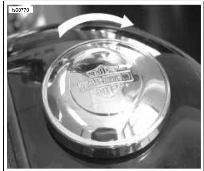
Figure 1. Right Hand Threaded Fuel Cap Installation
