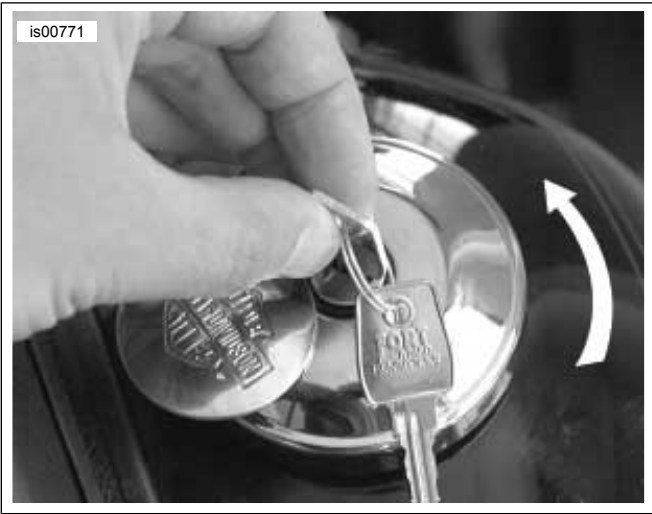
Figure 2. Right Hand Threaded Fuel Cap Removal
