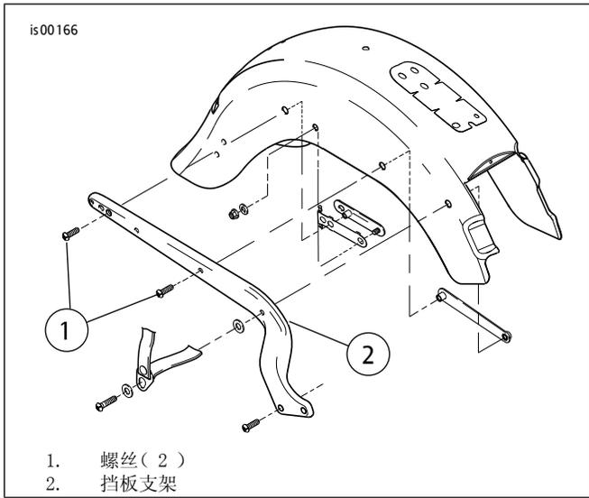
图1。拆卸螺丝 ( FLST/C/F )
