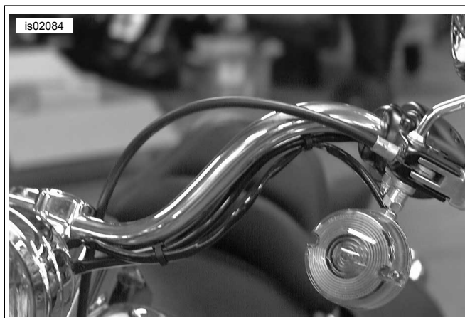
Figure 3. Clutch Cable Routing
