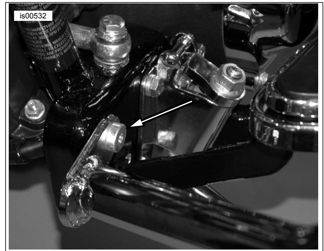
Figure 2. TORX Screw Removal (left side shown)
