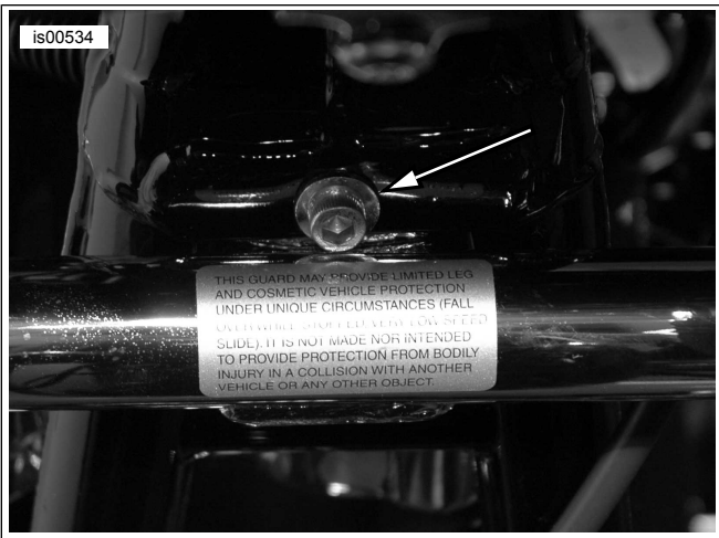
Figure 4. Hex Socket Head Screw and Washer Removal
