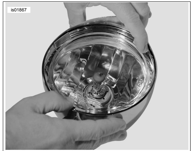
Figure 16. Chrome Trim Ring (two-sided tape shown)
