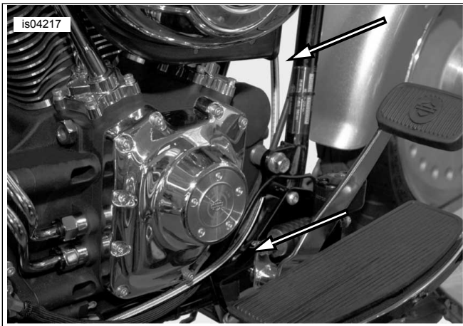
Figure 17. Routing from Left Frame Downtube to Engine Cam Cover
