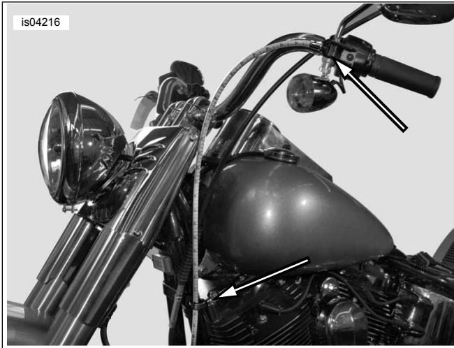
Figure 16. Routing from Hand Lever to Clamp at Left Frame Downtube
