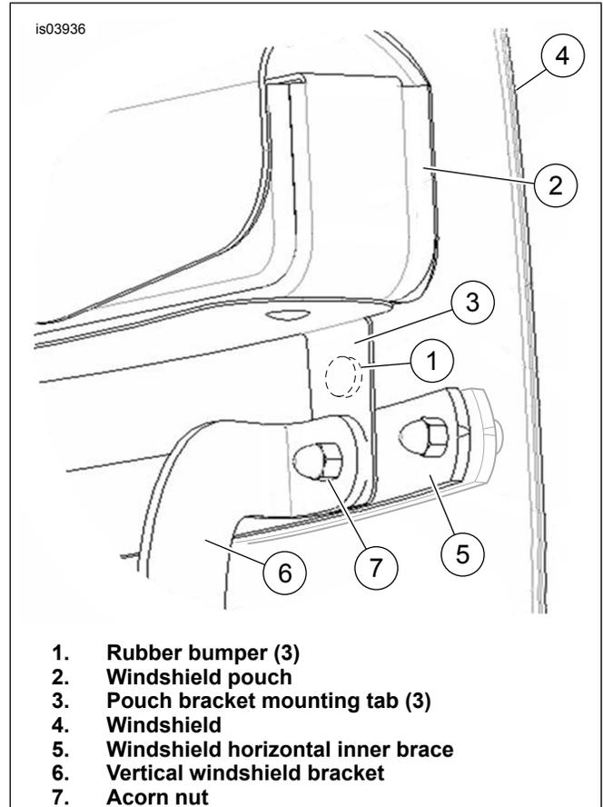
Figure 1. Windshield Pouch Installation, Side View
