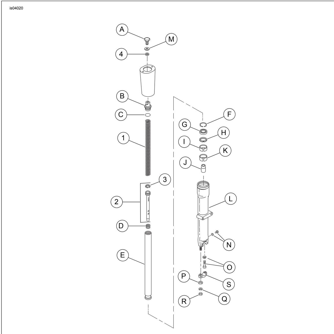
Figure 6. Service Parts: FL Softail Front Lowering Suspension Kit
