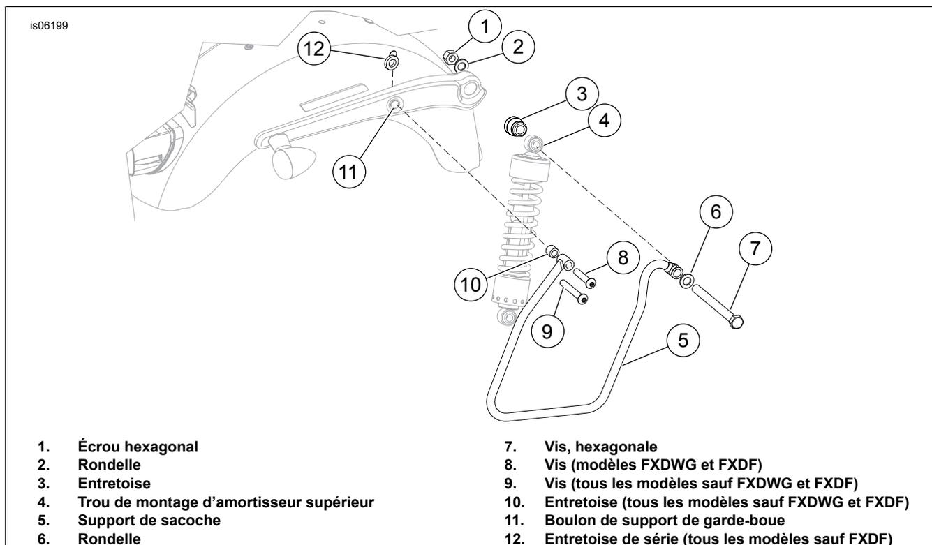
Figure 2. Installer le support de sacoches
