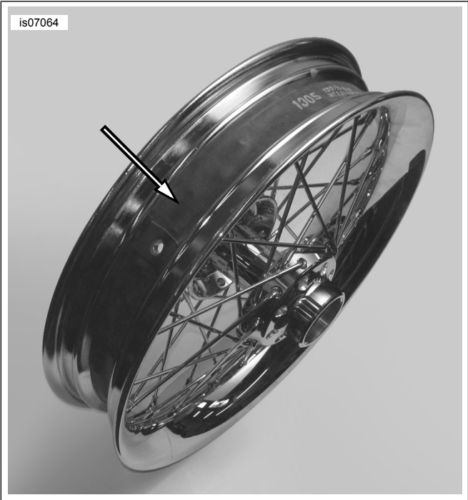
Figure 2. Installing Rim Strip, Tubeless Laced Wheel
