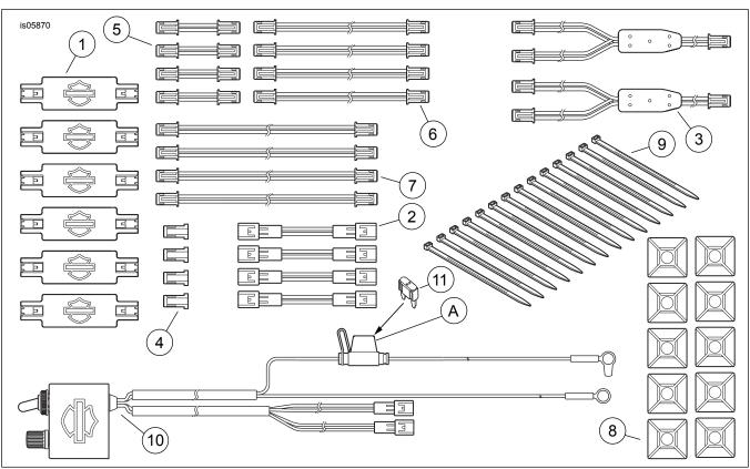
Figure 2. Service Parts, Electra-Glo Light Pod Kits
