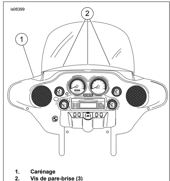
Figure 1. Installation du pare-brise
