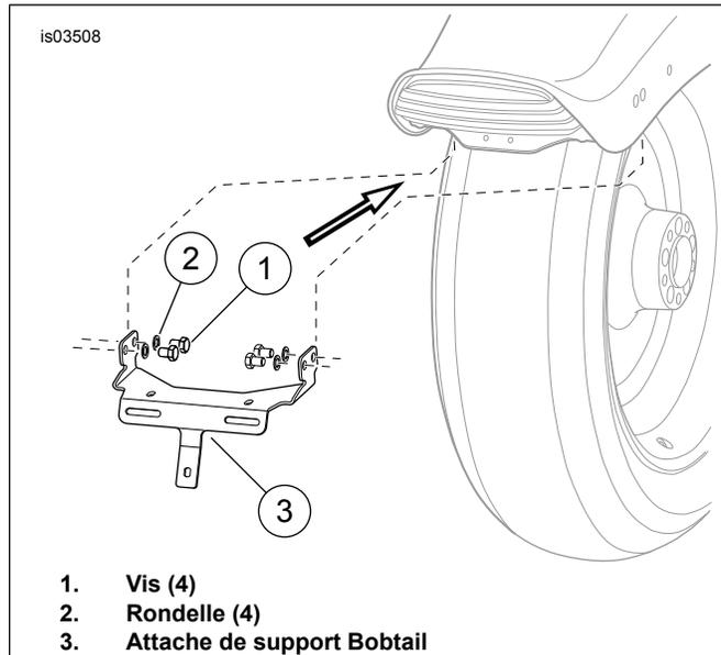
**Figure 4. Installation des attaches de support Bobtail**
