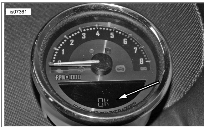
Figure 3. Speedometer Gauge Displaying "OK"
