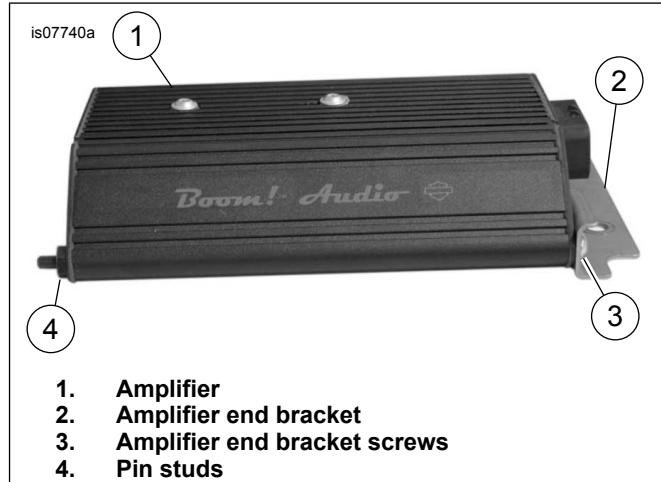
Figure 5. Amplifier Pin Studs and Amplifier End Bracket
