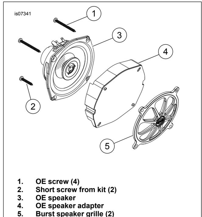
**Figure 1. Original Equipment (OE) Speaker Installation (Left Side Shown)**
