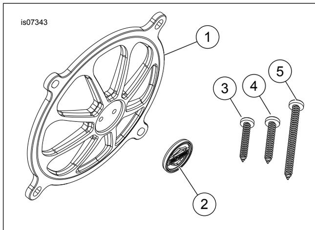
Figure 3. Service Parts: Burst Collection Speaker Grille
