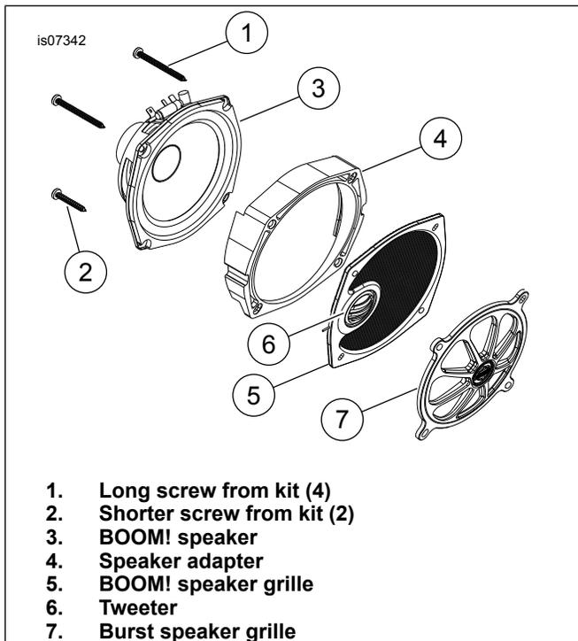
Figure 2. BOOM! Speaker Installation (Left Side Shown)
