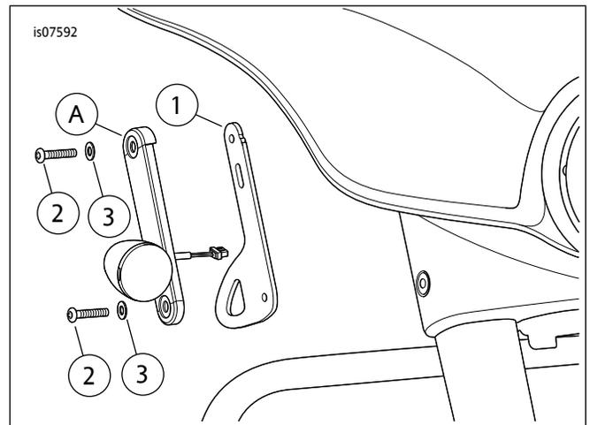
图1。安装捆绑带支架
