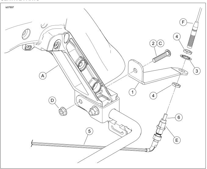
Figure 1. Service Parts, Antenna Relocation Kit
