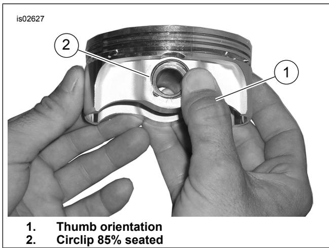
**Figure 4. Install Circlip**
