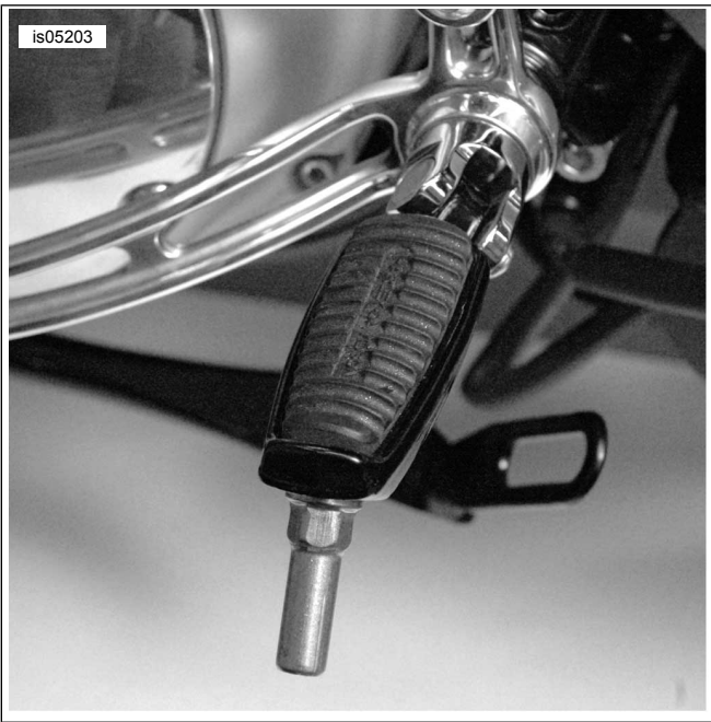
Figure 2. Correct installation (generic footpeg and wear tip)
