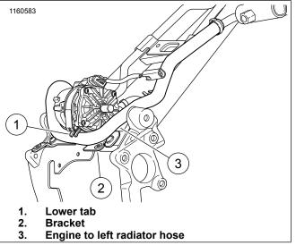
Figure 12. Positioning of Engine to Left Radiator Hose
