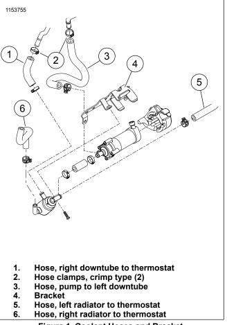
Figure 1. Coolant Hoses and Bracket
