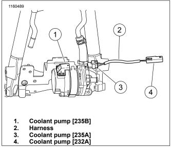
Figure 10. New Coolant Pump Harness
