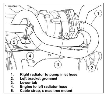
Figure 15. Routing of Right Radiator to Pump Inlet Hose
