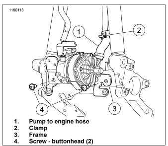
Figure 9. Installing Pump Assembly to Frame
