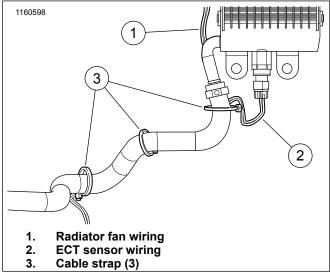
Figure 13. Securing Left Fan/ECT Sensor Wiring to Hose
