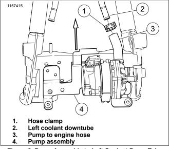
Figure 8. Pump Assembly to Left Coolant Down Tube
