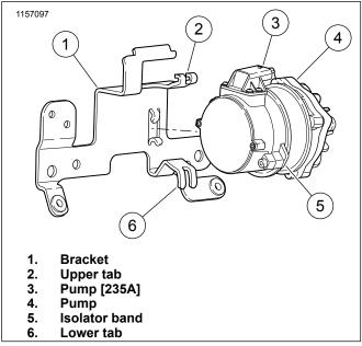
Figure 3. Pump and Bracket
