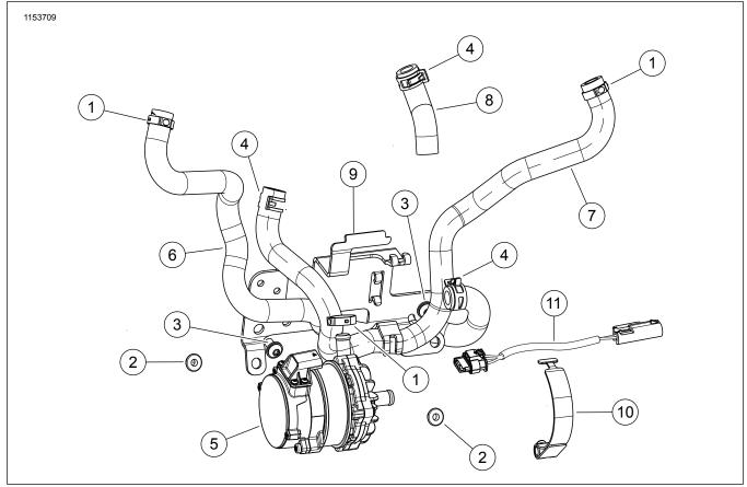
Figure 19. Service Parts: Coolant Pump System Kit
