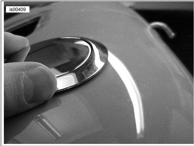
Figure 2. Determine Position for Trim Ring
