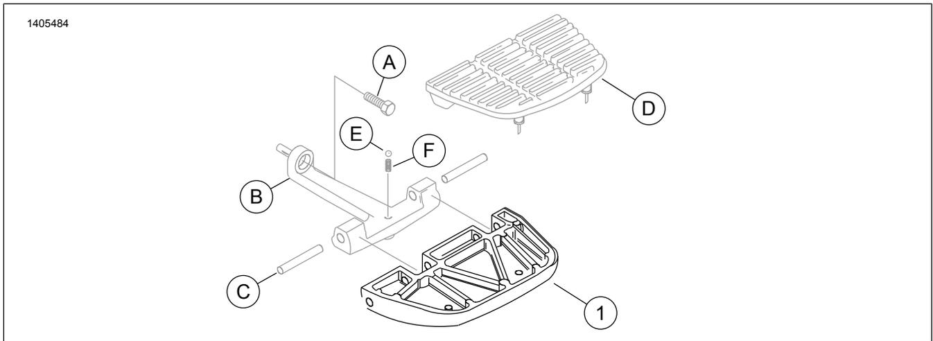
Figure 1. Kit Contents: Passenger Footboard Pan Kit Components
