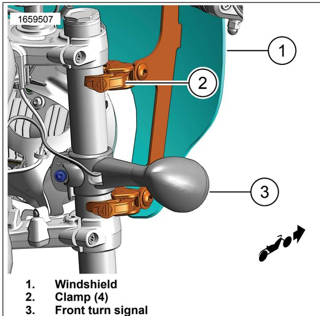
Figure 5. Windshield Installed
