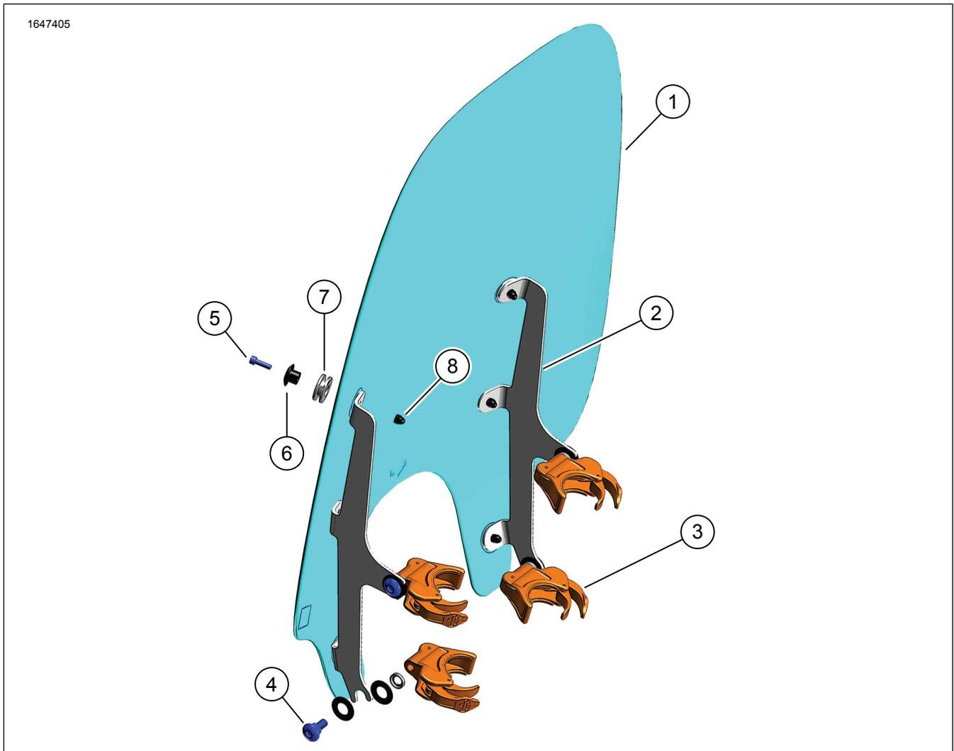
Figure 1. Kit Contents: Quick Release Windshield (Typical)
