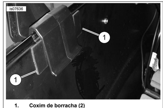
Figura 2. Instale coxins de borracha no interior do Tour-Pak
