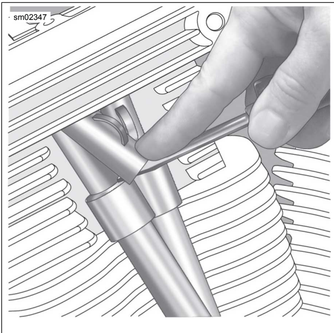
Figure 5. Install Spring Cap Retainers
