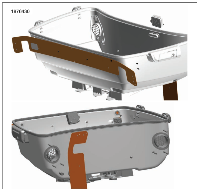
Figure 2. Placement du gabarit
