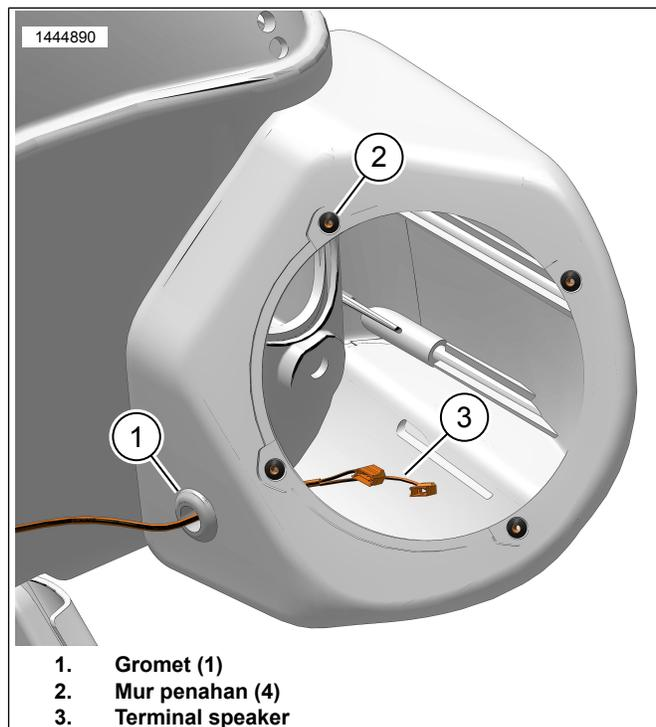
**Gambar 1. Harness Kabel Pod Speaker (Menampilkan Sisi Kiri)**
