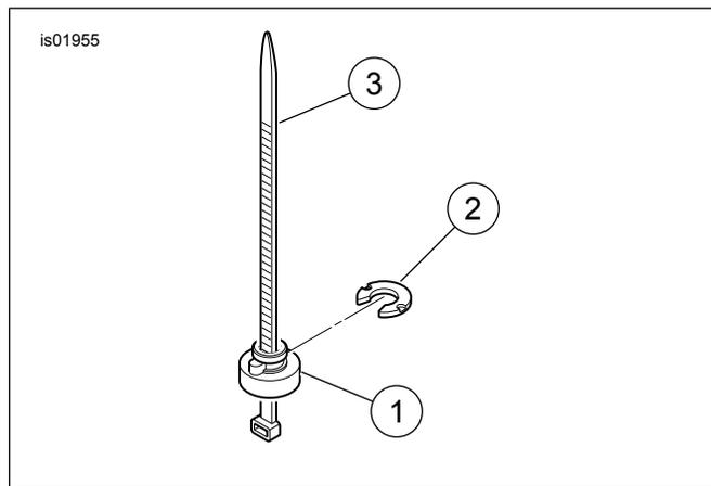
Figure 2. Installation Tool
