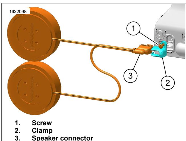
Figure 2. Disassembly
