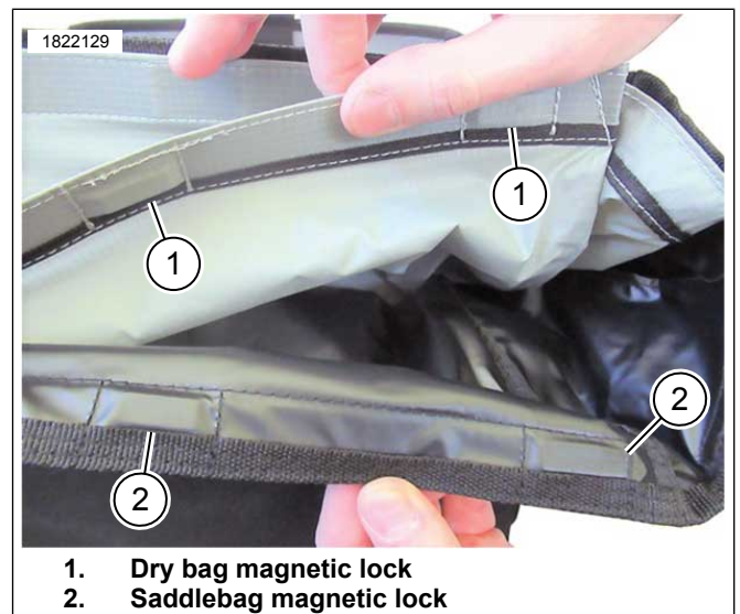
Figure 12. Dry Bag Install
