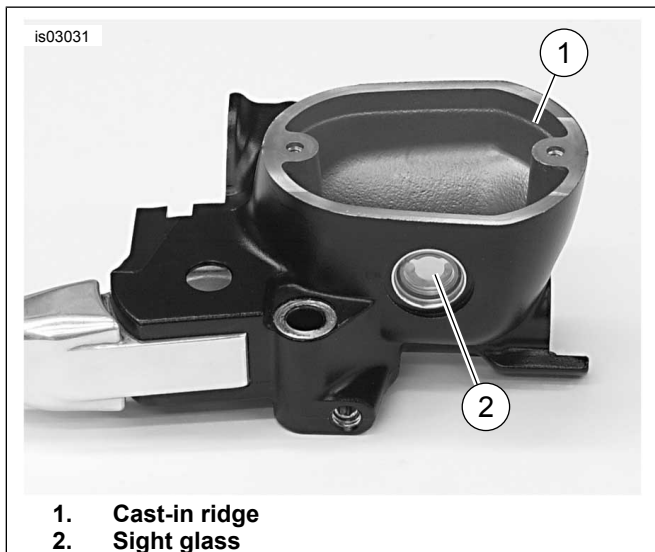
Figure 6. Filling Front Master Cylinder Reservoir
