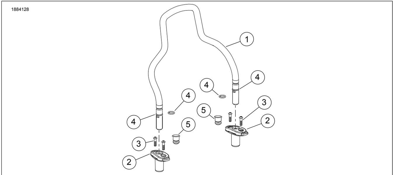
Figure 1. Kit Contents: Quick-Release Sissy Bar Upright Kit
