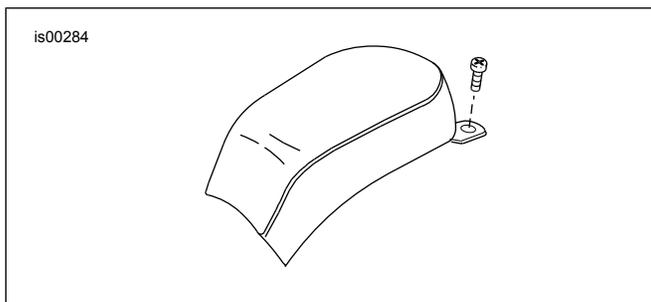
**Figura 2. Remover o parafuso**
