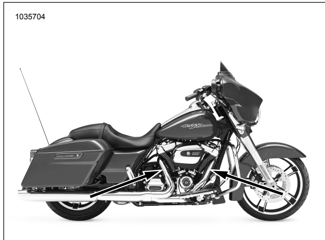
Figure 11. Oxygen Sensor Locations (Inboard Side of Exhaust Pipes)
