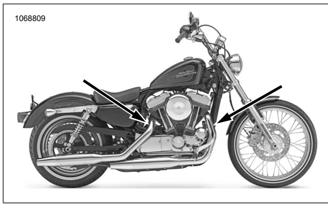
Figure 48. Oxygen Sensor Locations (Inboard Side of Exhaust Pipes)
